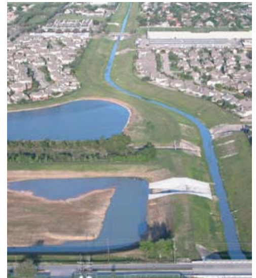
The Old Westheimer Stormwater Detention Basin can hold approximately 200 million gallons of stormwater.
