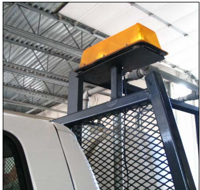
Newly Installed Safety Light
